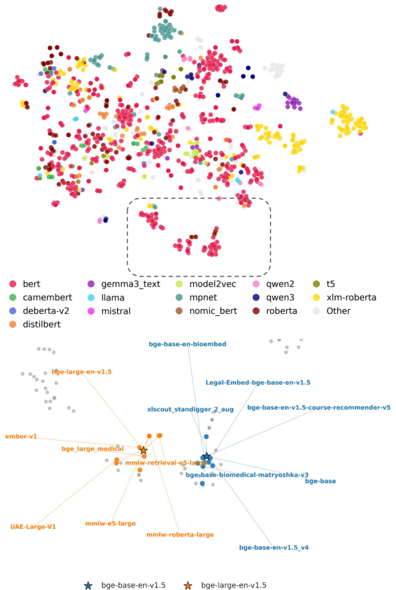
Figure 1: Map of Encoders. Top: Map for 1101 sentence encoders, visualised by t-SNE and coloured by the encoder type. Bottom: A 30% zoomed-in view of the dotted area showing the top-7 nearest neighbours for bge-base and bge-large . Nearest neighbours belong to the same primary architecture and are closely located.
